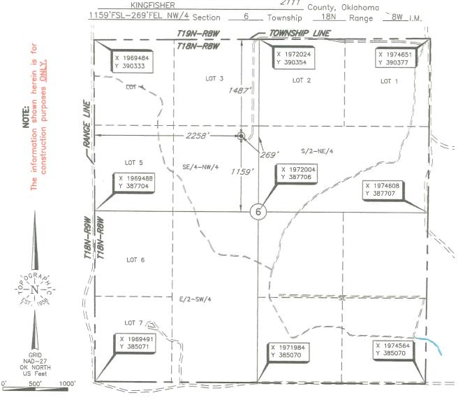
Operator: BROWN & BORRELI, INC. **ELEVATION:** Lease Name: DAN 1100' Gr. at Old Pad Well No.: 1-6 Topography & Vegetation Existing Well Loc. fell in Pasture Land with Brush Reference Stakes or Alternate Location Good Drill Site? YES Stakes Set <u>NON</u>E Best Accessibility to Location From North off Lease Road Distance & Direction from Hwy Jct or Town From St. Hwy 51& Lacey, OK- Go South ±3 miles to the NE corner of Sec 6-T18N-R8W
