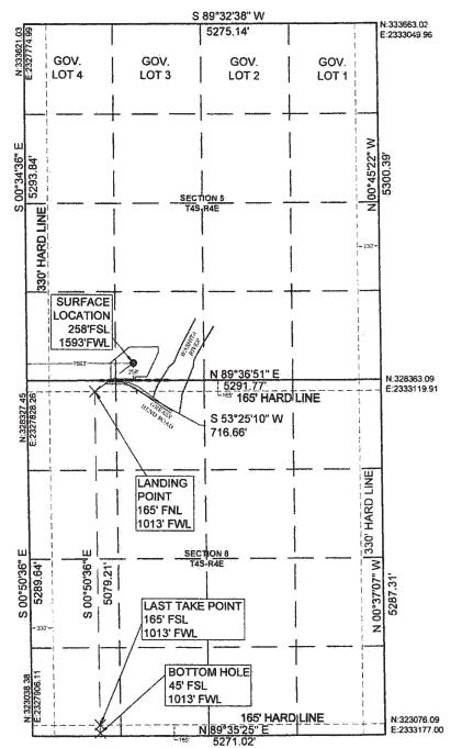
NAD 27 OK SOUTH SURFACE LOCATION 34.231407°N LAT: LONG: 96.910154°W N= 328596.39' E= 2329419.15 LANDING POINT N= 328169.3° E= 2328843.66 LAST TAKE POINT N= 323210.67' E= 2328916.61 **BOTTOM HOLE** N= 323090.68' E= 2328918.37'
