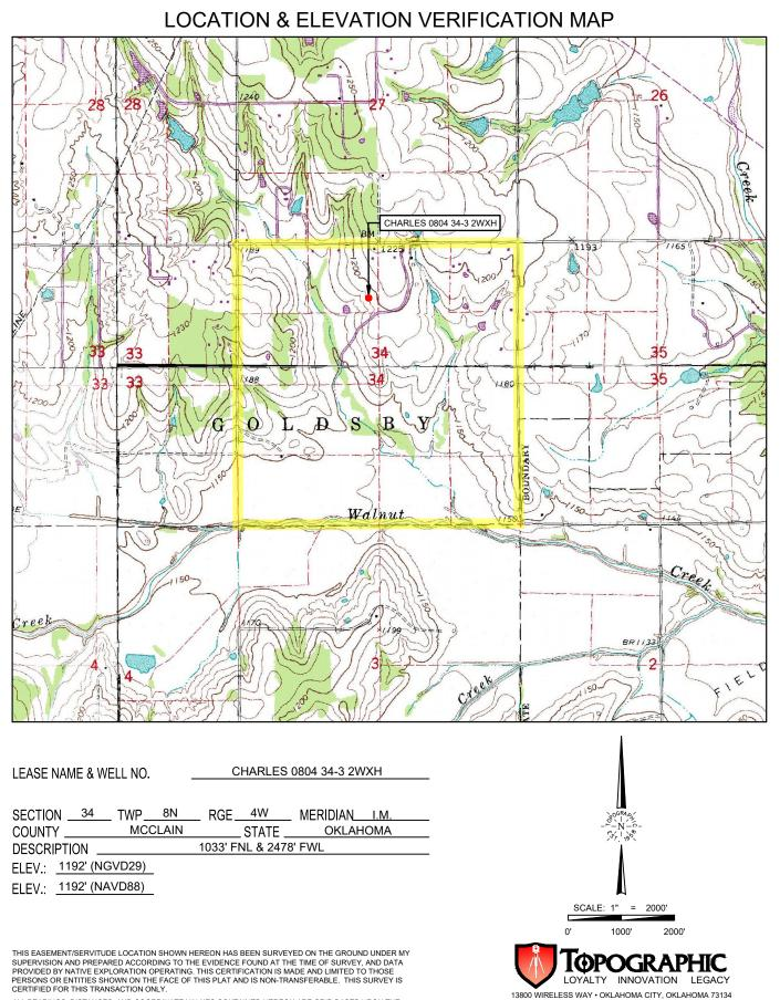
ALL BEARINGS, DISTANCES, AND COORDINATE VALUES CONTAINED HEREON ARE GRID BASED UPON THE OKLAHOMA STATE PLANE COORDINATE SYSTEM, SOUTH ZONE OF THE NORTH AMERICAN DATUM, U.S. SURVEY FEET.
