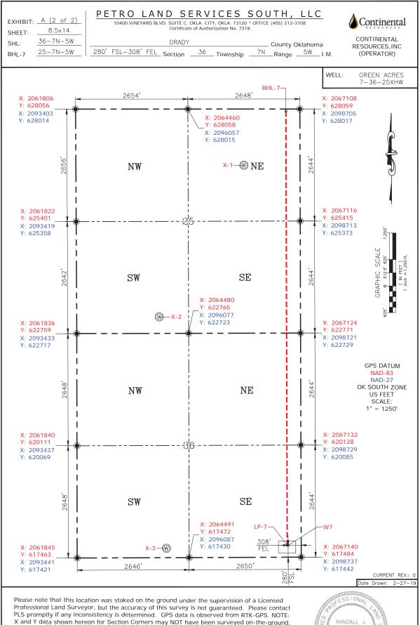
X and Y data shown hereon for Section Corners may NOT have been surveyed on-the-ground, and further, does NOT represent a true Boundary Survey. Quarter Section distances may be assumed from a Government Survey Plat or assumed at a proportionate distance from opposing section corners, or occupation thereof, and may not have been measured on-the-ground, and further, does not represent a true Boundary Survey.
