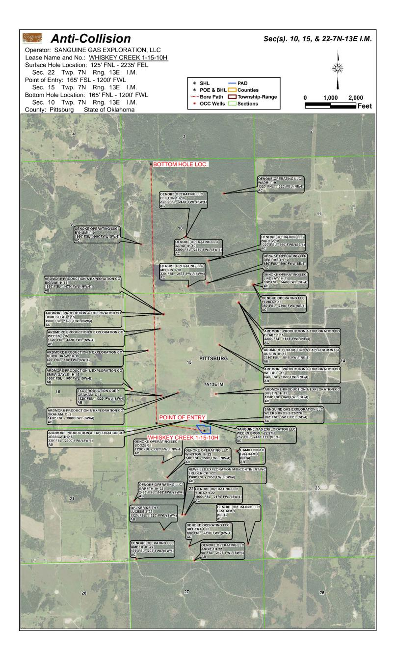
Operator: SANGUINE GAS EXPLORATION, LLC Lease Name and No.: <u>WHISKEY CREEK 1-15-10H</u> Surface Hole Location: 125' FNL - 2235' FEL Sec. 22 Twp. 7N Rng. 13E I.M. Point of Entry: 165' FSL - 1200' FWL Sec. 15 Twp. 7N Rng. 13E I.M. Bottom Hole Location: 165' FNL - 1200' FWL Sec. 10 Twp. 7N Rng. 13E I.M. County: Pittsburg State of Oklahoma Ground Elevation at Surface Hole Location: ±781'
