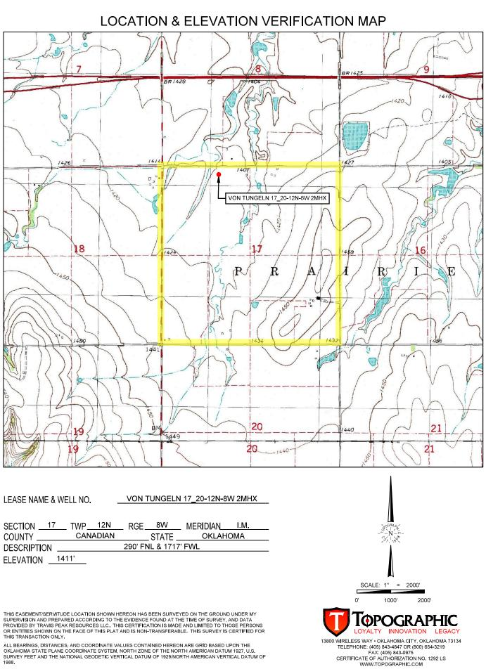
OKLAHOMA STATE PLANE COORDINATE SYSTEM, NORTH ZONE OF THE NORTH AMERICAN DATUM 1927, U.S. SURVEY FEET AND THE NATIONAL GEODETIC VERTICAL DATUM OF 1929/NORTH AMERICAN VERTICAL DATUM OF 1988.
