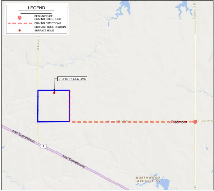
STEPHEN 1406 5H-27X LEASE NAME & WELL NO. SECTION 27 TWP 14N \_ MERIDIAN\_\_\_ 6W RGE\_ COUNTY \_\_\_\_ CANADIAN STATE OKLAHOMA 410' FNL & 2435' FEL DESCRIPTION **DISTANCE & DIRECTION** FROM PIEDMONT, OK GO ±4.0 MI. WEST ON EDMOND RD. NW, THEN GO ±1.0 MI. NORTH ON CIMARRON RD. NW TO THE NORTHEAST CORNER OF SECTION 27-T14N-R6W.
