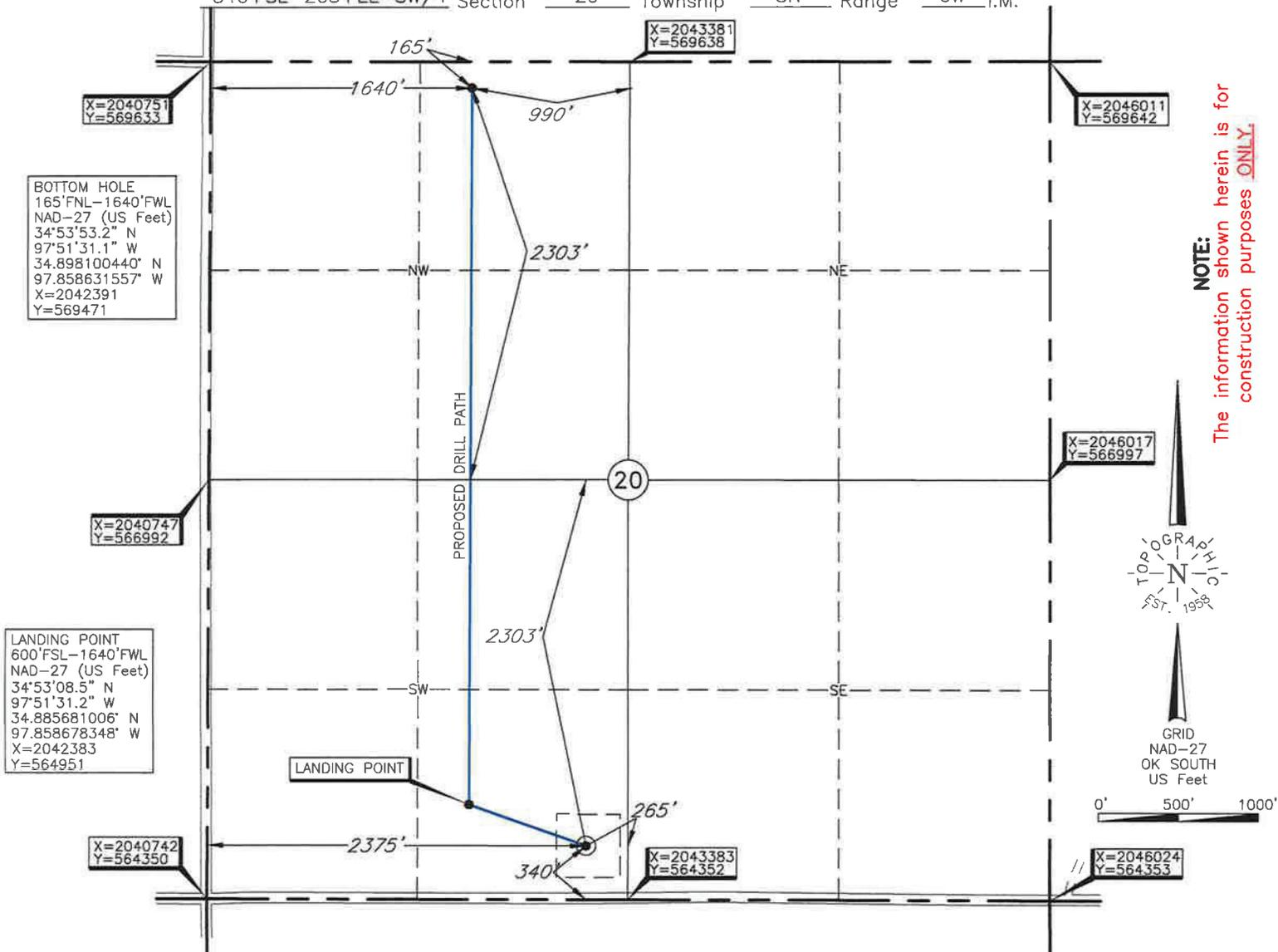
LANDING POINT, BOTTOM HOLE AND DRILL PATH INFORMATION PROVIDED BY OPERATOR LISTED, NOT SURVEYED.
