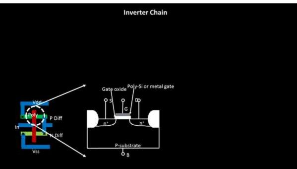
If we go by **ideal fabrication process**, below is what you will achieve, a perfectly cubic shape (below is the 2D image, so it looks rectangle) oxide layer, and perfectly deposited metal gate or poly-silicon gate
