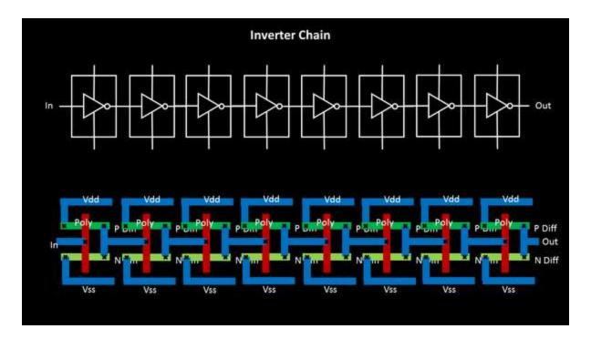
We use photo-lithography fabrication technique to build the inverters on Silicon wafer, and this is a non-ideal process, where the edges will not exactly be straight lines, but there will be disturbances.
