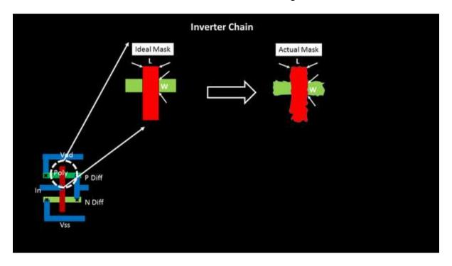
Now these variations on the sides, is also dependent on **what logic cell is present on either side of this inverter**, if its surrounded by chain of inverters on either side, the variation on the sides will be less as the process parameters to build mask for a chain of similar size inverter, is almost the same.
