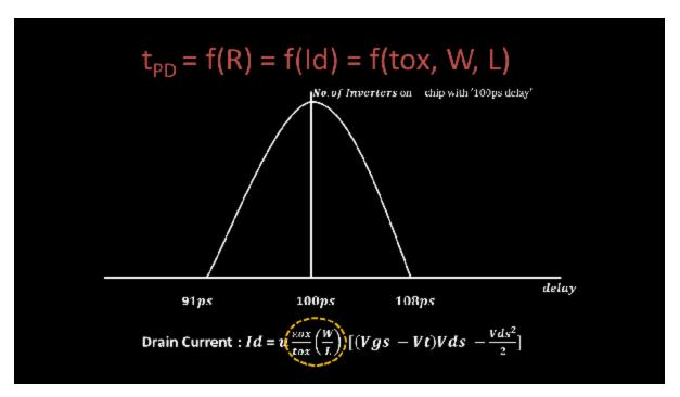
Now, we know the percentage variation in delays of inverter compared to '100ps', because that's where the inverter delay (with used 'W/L' ratio) is expected to be, and most number of inverters on chip with that 'W/L' ratio have a delay of 100ps
