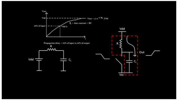
With above, we can safely say, the propagation delay tPD is a function of 'R'
