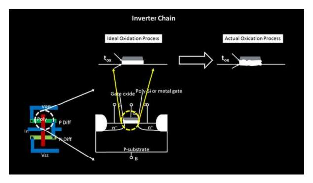
So, what's wrong having above oxide thickness. Again, it's the drain current (which is a function of oxide thickness, shown in below image) that will get varied for the complete chain of inverter, especially, the one's on the sides. The variations in middle inverters will still be uniform. We discussed the reason for this in last post
