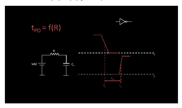
Now, from previous posts, we seen variation in drain current 'Id' due to variation in 'W/L' and 'oxide thickness' variations, and above we see, how propagation delay is function of 'R'.
