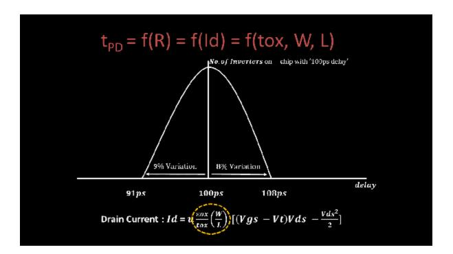
OCV variation is +8% and -9% and one of them will be used for launch and other for capture in setup/hold timing calculations.
