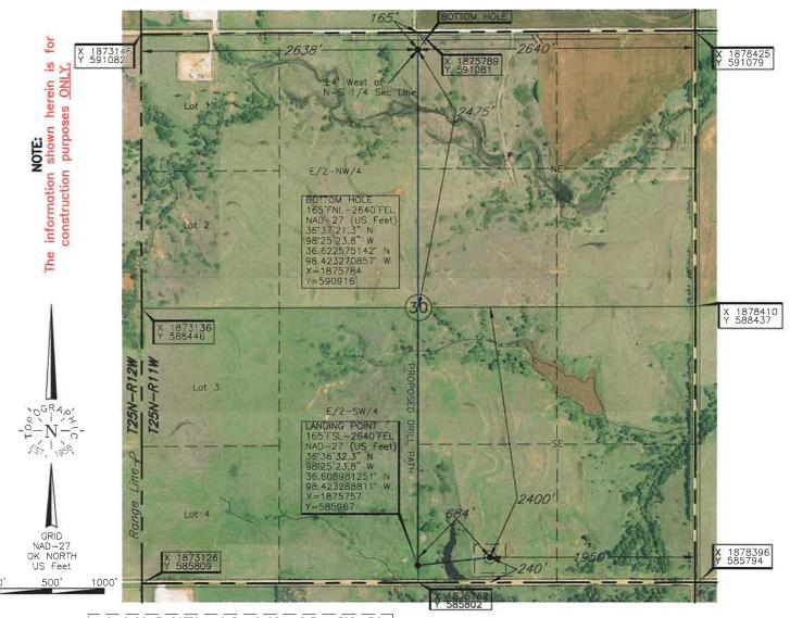
LANDING POINT, BOTTOM HOLE AND DRILL PATH INFORMATION PROVIDED BY OPERATOR LISTED, NOT SURVEYED.
