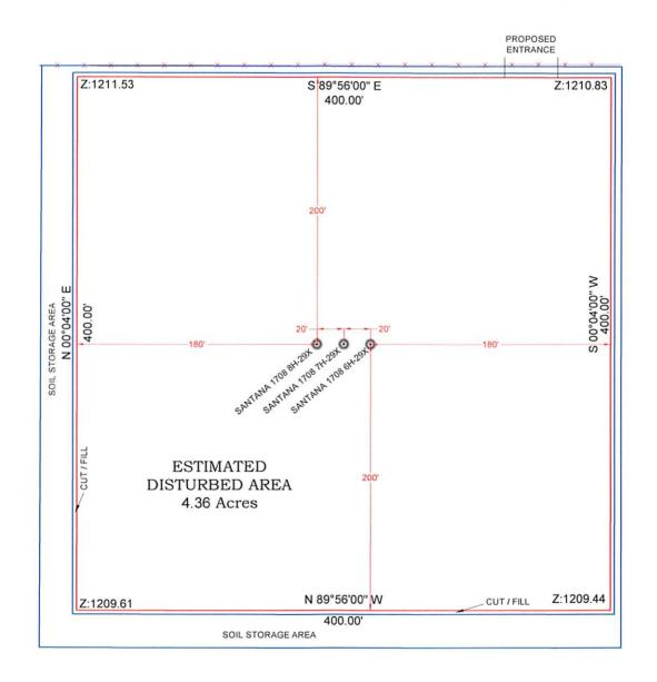
ELEVATIONS SHOWN ARE DERIVED FROM AN OPUS OBSERVATION AND ARE IN U.S. SURVEY FEET NORTH AMERICAN VERTICAL DATUM 1988 (NAVD88).
