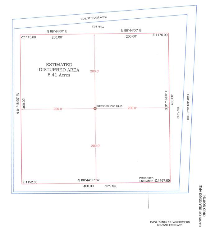
TOPO POINTS AT PAD CORNERS SHOWN HERON ARE INTERPOLATED FROM USGS QUADRANGLE AND HAVE NOT BEEN FIELD VERIFIED
