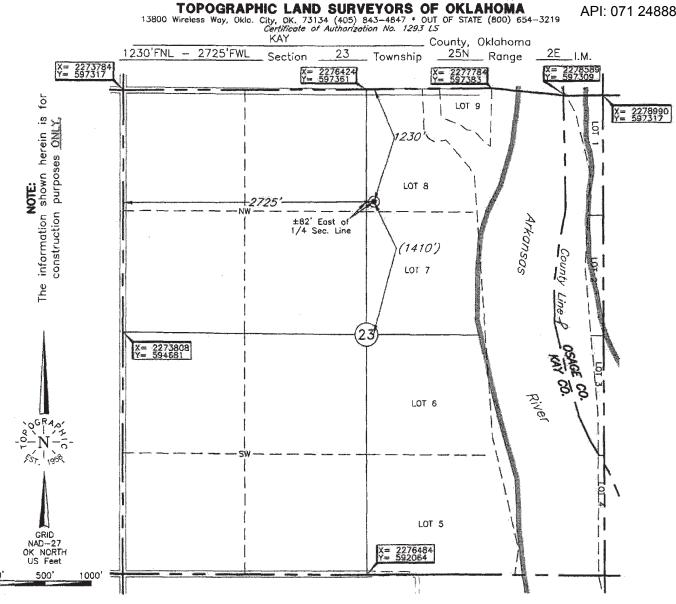
Distances shown in (parenthesis) are calculated based upon the Quarter Section being 2640 feet, those shown in [brackets] are based on GLO (General Land Office). distances and have NOT been measured on the ground.
